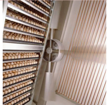
Separate heating, cooling and ventilation controls per incubator section of 19,200 hen eggs.
